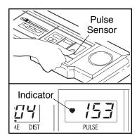
indicator in the pulse display flashes **steadily**. Hold your thumb at this level. After a few seconds, three dashes will appear in the display and your pulse will be shown. Hold your thumb on the sensor for another 15 seconds for the most accurate reading. If the displayed pulse appears to be too high or too low, or if your pulse is not displayed, lift your thumb off the sensor and allow the display to reset. Press down again on the sensor as described above.
